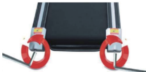
Figure B Adjustment Method for Walking Belt Deviating to the Right
